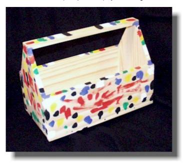
**Step 1** - Purchase a pine "Project Panel" 12"x36" to cut pieces from. Project panels are approx. 3/4" thick glued pine strips to form a board for wood projects. (Available at home centers) Other materials needed will be wood glue, and 6d nails.
